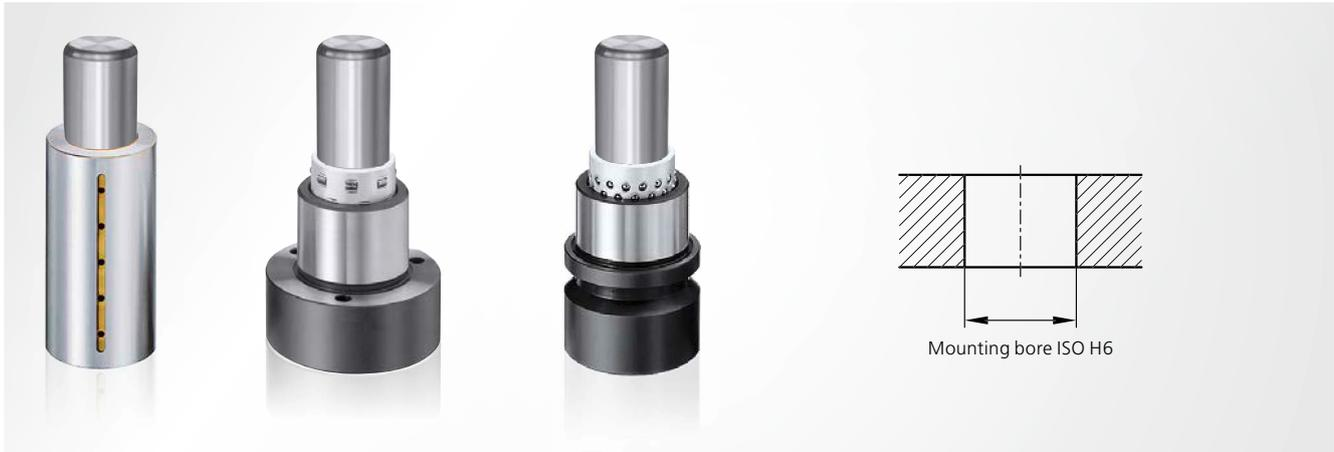
The highly-precise guide units from STEINEL are used in toolmaking, fixture manufacturing and machine engineering. The range includes three types of sliding guide (bronzed steel, with solid lubricant and solid lubricant rings) and two types of roller guide (roller and ball guides).
