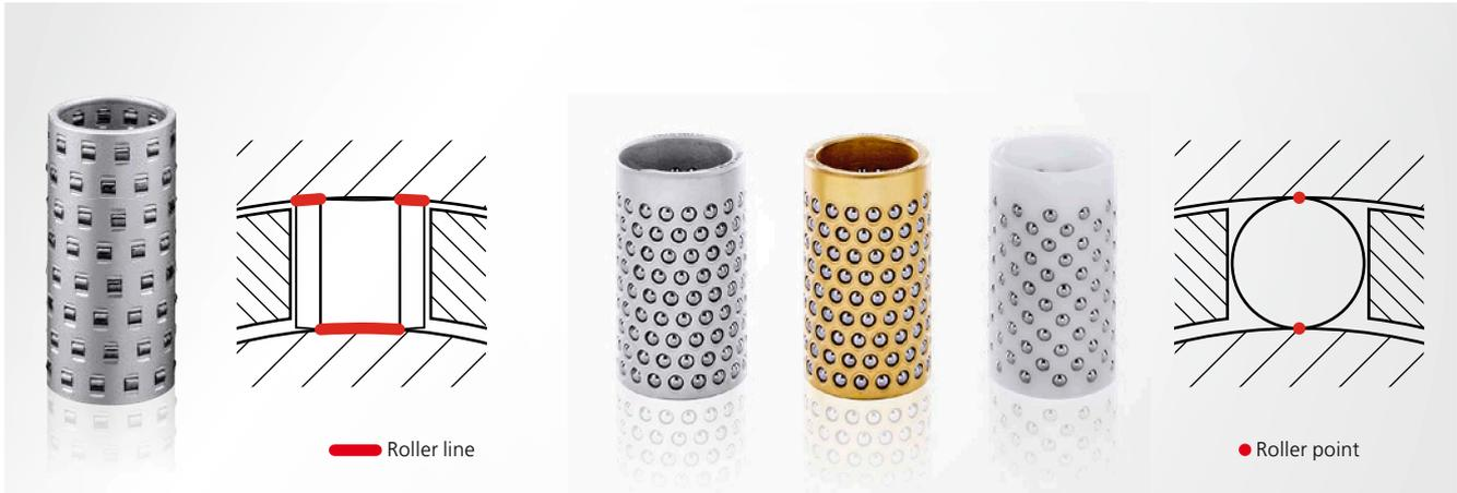
STEINEL roller guides (roller and ball guides) consist of a guide pillar, a roller or ball guide and a guide bush, which are paired together free of clearance. The cage travel is only half as long as the stroke of the guide.
